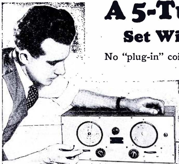
To the left is shown the new Hallcrafters compact "loud-speaker" S-W receiver in operation. "Regen." control at right.
