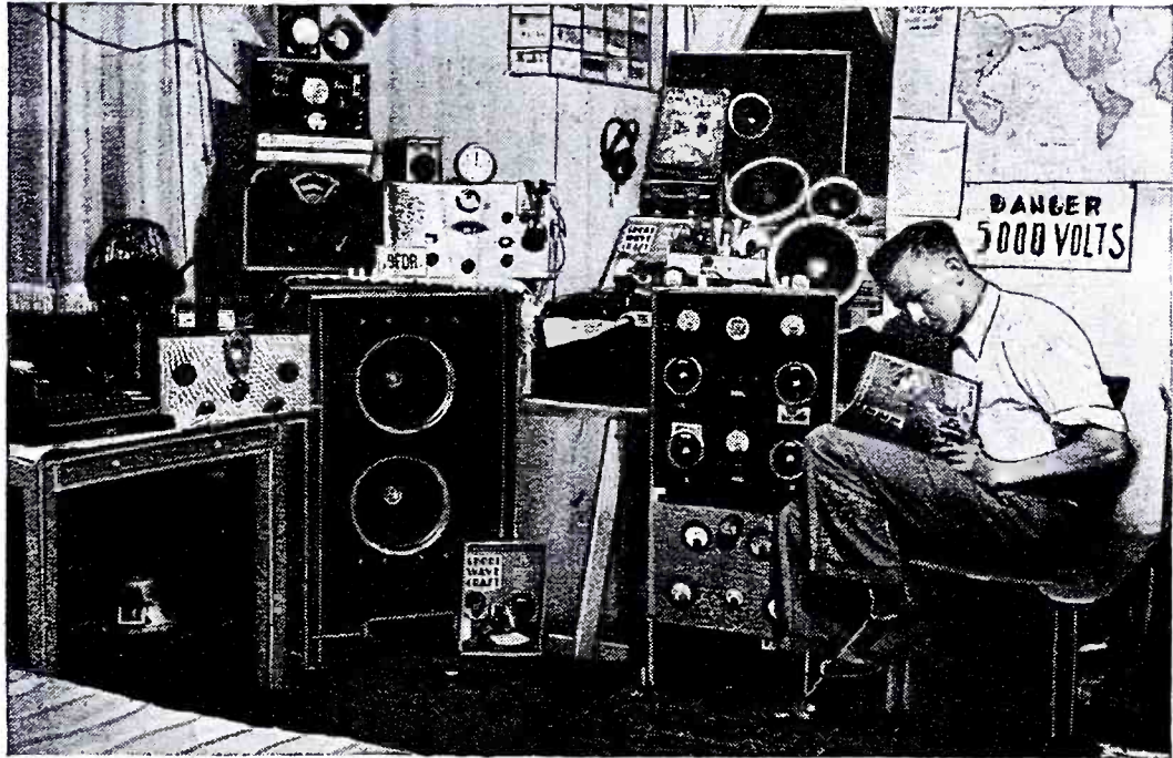
Max Fiegen has a very fine short-wave station which boasts an elaborate array of apparatus, including a 11-tube short-wave receiver and also a 5 and 10-meter set.
